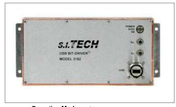
Operation Mode: USB 2.0 Input/Output Interface: USB Type B
